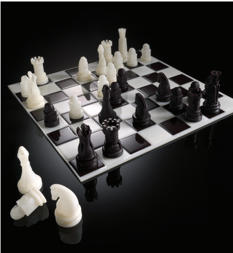
Parts made with new RenShape® SL 7820 photopolymer.
